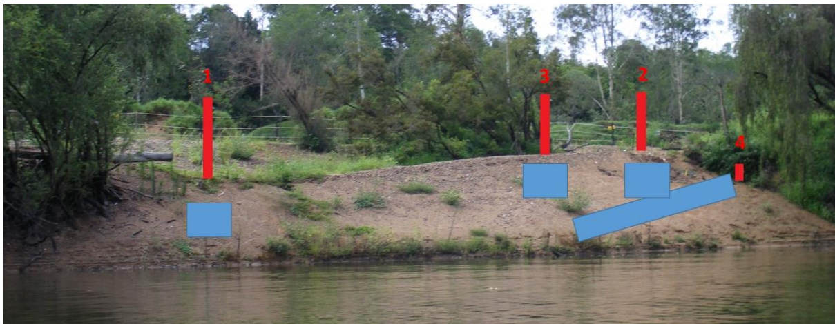
Fig. 6. Four wild life camera posts (red) and their area of view (blue)
