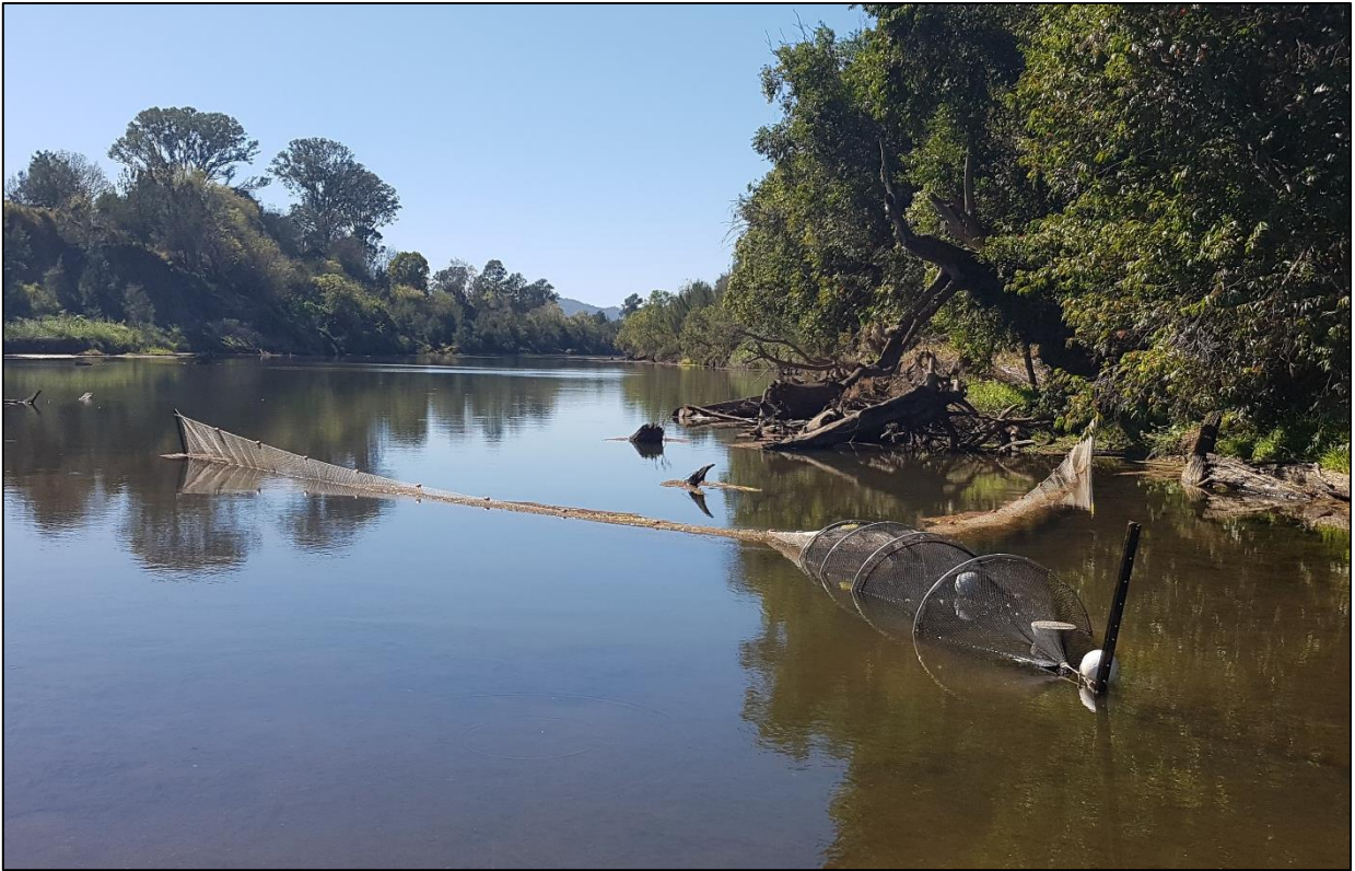
Figure 4: Double-winged set net deployed at a site in the mid catchment (Ka5).
